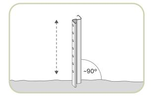
1. Set the post vertically and watch the plumb line while hammering the post into the ground.
